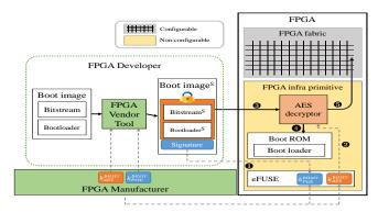
Figure 1: A generic secure boot architecture of FPGA
